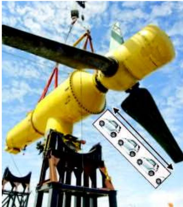
Tidal Generation Ltd's prototype tidal turbine waiting to be deployed at the European Marine Energy Centre, Scotland.
